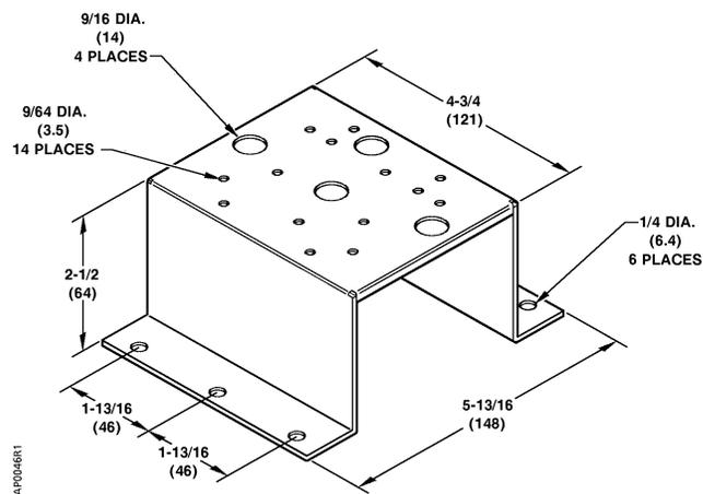
**Figure 10. Offset Mounting Bracket 333-176.
