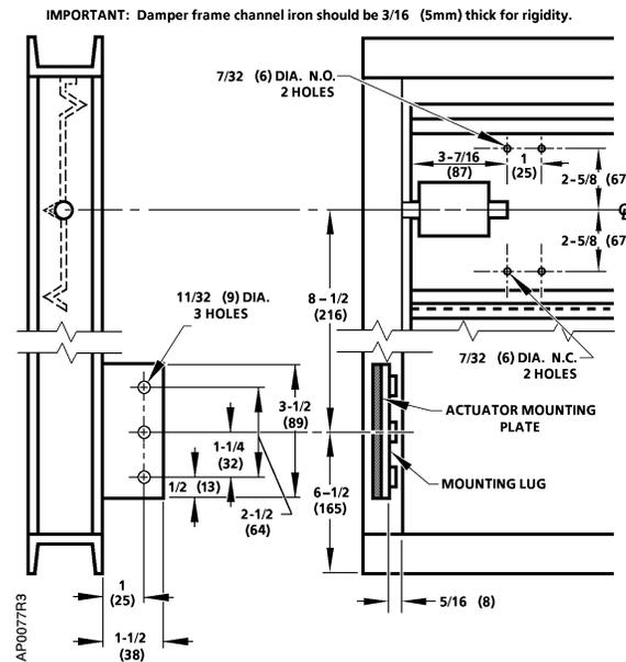
**Figure 4. Frame Mounting Dimensions in Inches (Millimeters).**
