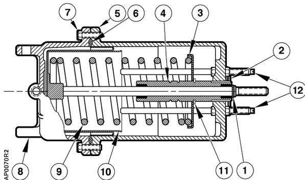
**Figure 1. Standard Actuator.**
