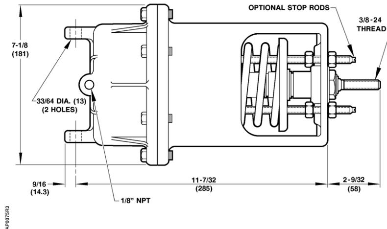
**Figure 9. Extended Shaft Remote Mounting with Travel Stops.
