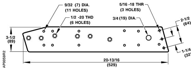
**Figure 11. Actuator Mounting Plate 331-623.
