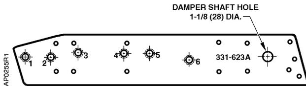
**Figure 8. Actuator Mounting Plate 331-623A Pivot Shaft Locations.**
